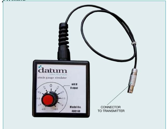
Please note that it is only possible to use the strain gauge simulator whilst the shaft is static as you will need to connect to the on shaft transmitter.
