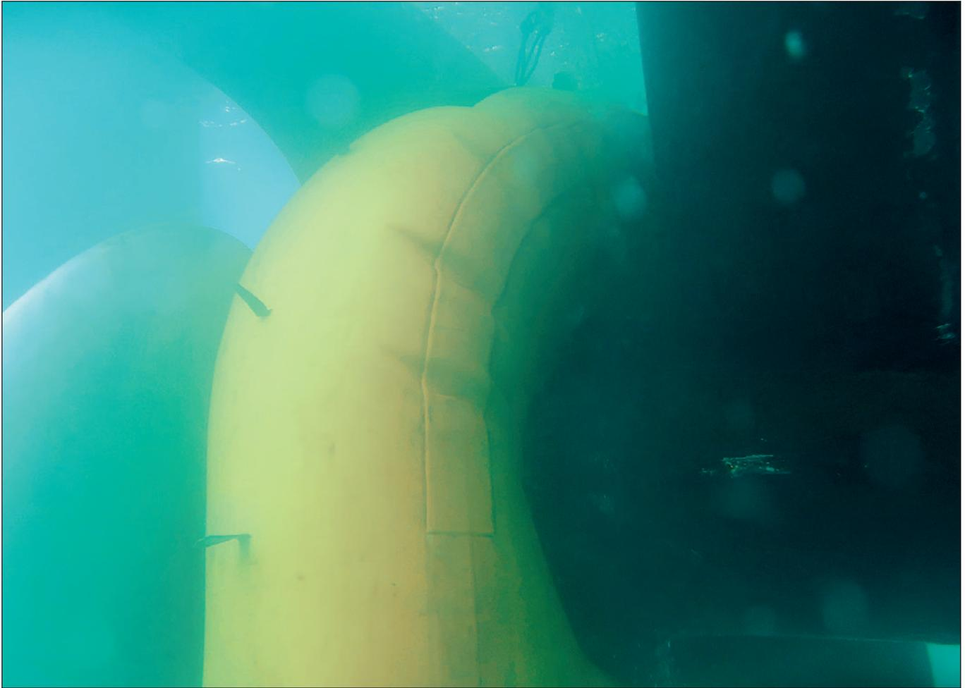
**U**sing our flexible mobdock method to create a dry underwater environment, we have carried out stern tube seal repairs and replacements underwater for some years now in cooperation with OEMs.
