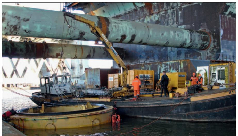
*A special ring mobdock was used to seal off the compartment of the thrusters of a large crane vessel.*
