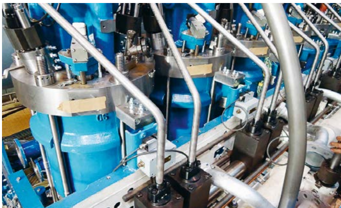
Common-rail system on Wärtsilä X35 engine.
