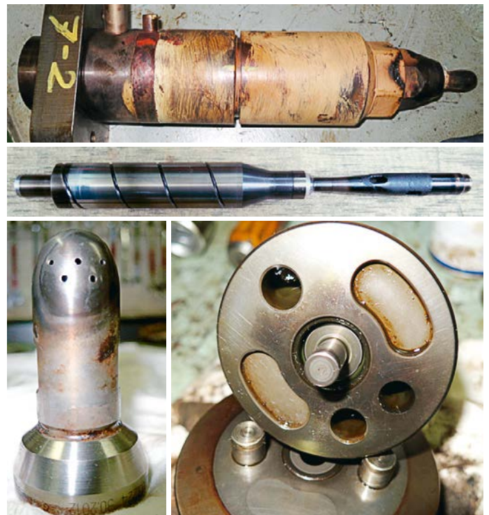
Different components of FAST injector inspected after 12'600 rhs.
