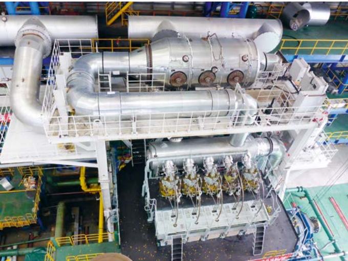
SCR Pilot Project 5RT-flex58T-D.
