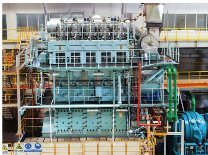
Wärtsilä 5RT-flex50DF with Turbocharger at the aft end.
