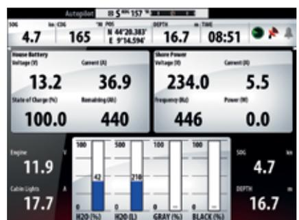
**CZone** integration - battery and tank monitoring
